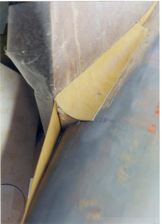
PLYWOOD FILETT WAS ADDED TO THE FUSE AFTER IT WAS FIBERGLASSED
